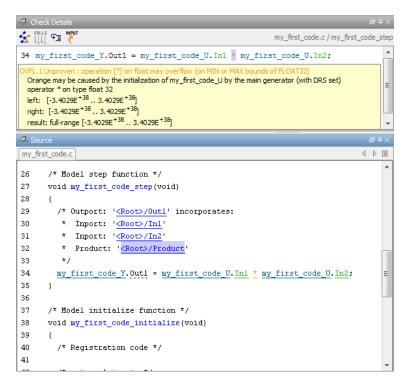
This orange check shows a potential overflow issue when multiplying the signals from the inports In1 and In2. To fix this issue, you must return to the model.
